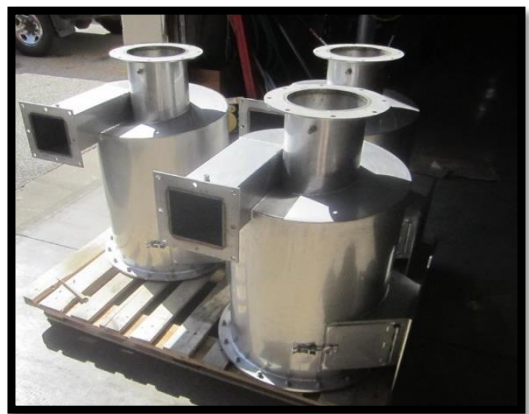
Stainless Steel GPC Cyclone
